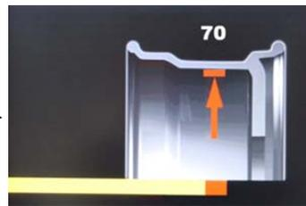
Pull the sensor arm and stick the counterweight on the exact "0" distance position shown on the inside display window
